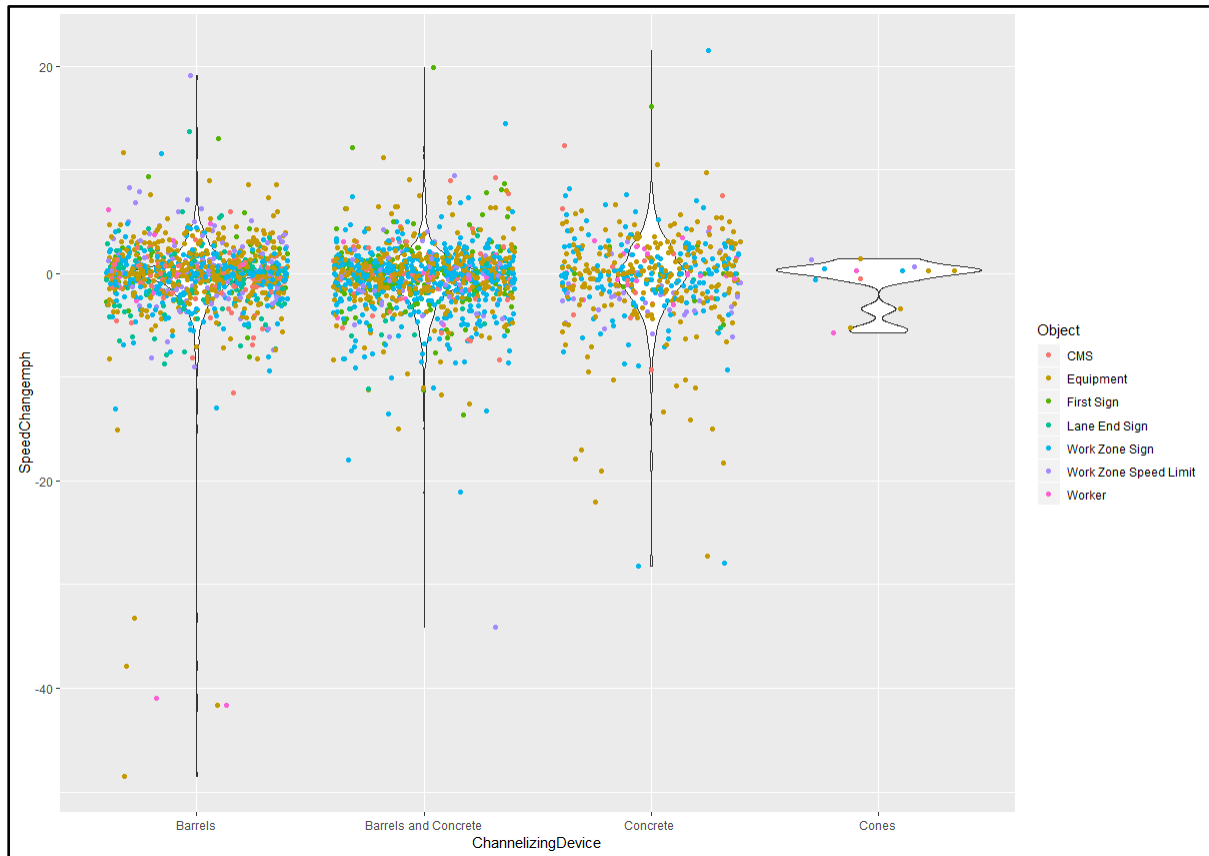
Figure 5-4 Change in Speed for Channelizing Devices
